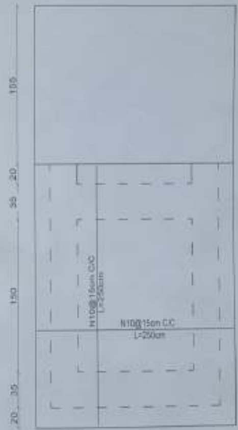
Second Floor Slab Rebar Plan
