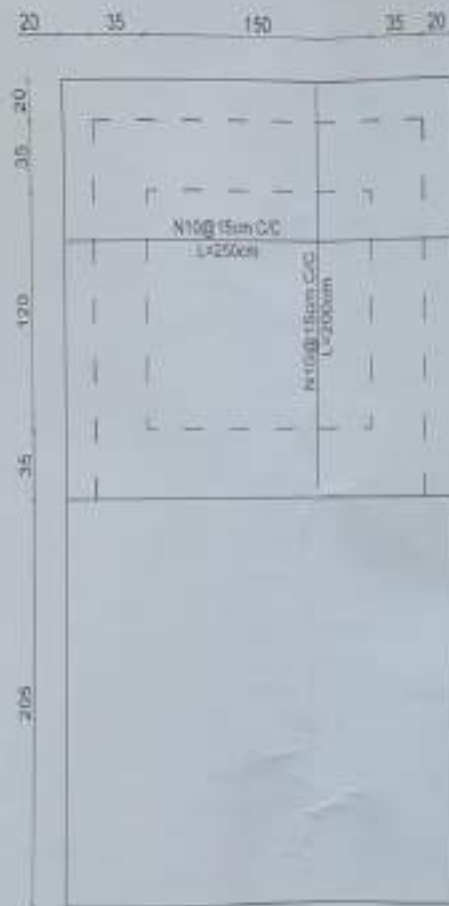
Second Floor Slab Rebar Plan
