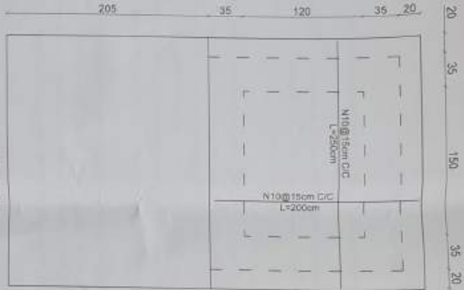
Second Floor Slab Rebar Plan
